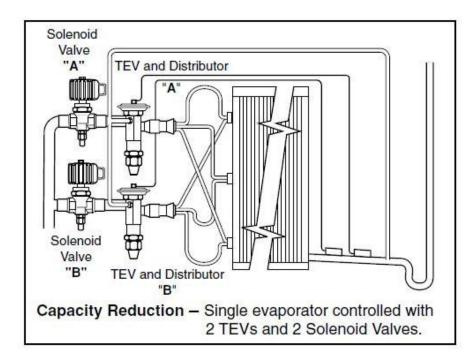
Capacity is accomplished by closing a solenoid valve which deactivates the circuits being fed by the TEV and distributor downstream of the solenoid valve. This method of capacity control, however, requires a degree of care since the heat load on the evaporator circuits will be affected in the manner In which circuits are deactivated
